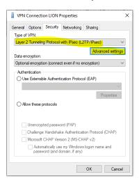
Select in the pulldown menu <Type of VPN> Layer 2 Tunneling Protocol with IPsec (L2TP/IPsec)
